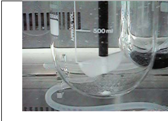
shows degassed media - no floating particles particles if properly degassed
